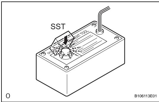
(2) Press the SST activation switch and check that the LED of the SST activation switch illuminates.
