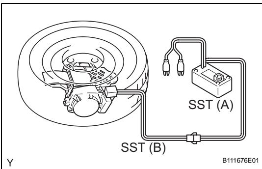
(2) Place the front seat outer belt on the ground and cover it with a tire (with wheel).
