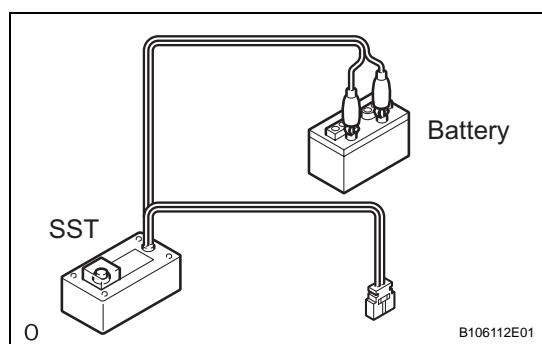
(1) Connect SST's red clip to the battery's positive (+) terminal and the black clip to the battery's negative (-) terminal.
