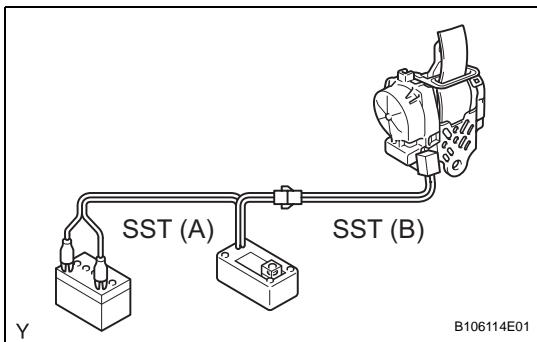
(2) Connect SST (A) to SST (B). Then connect SST (B)'s connector to the seat belt pretensioner.
